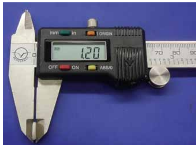
Fig. 1: Lithium disilicate disk after layering showing thickness of 1.2 mm
